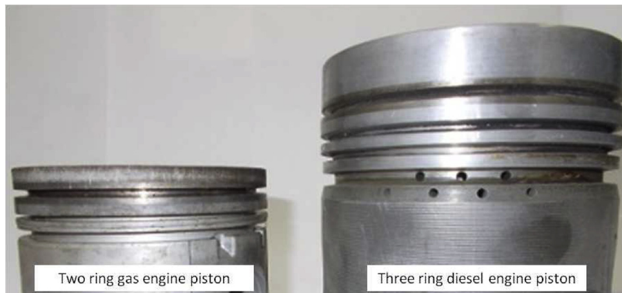
Fig. 8 – Number of rings on typical gasoline and diesel engine pistons.
